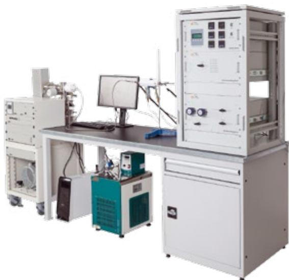
Example of a custom designed sorption system that contains software controlled conditioning units for up and down stream, sorption and gas analysis unit
