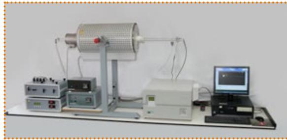
Example of a custom designed catalyst screening test system that contains software controlled conditioning units for up and down stream, two zone temperature controlled reactor, which can be adjusted both vertical and horizontal, and gas analysis unit
