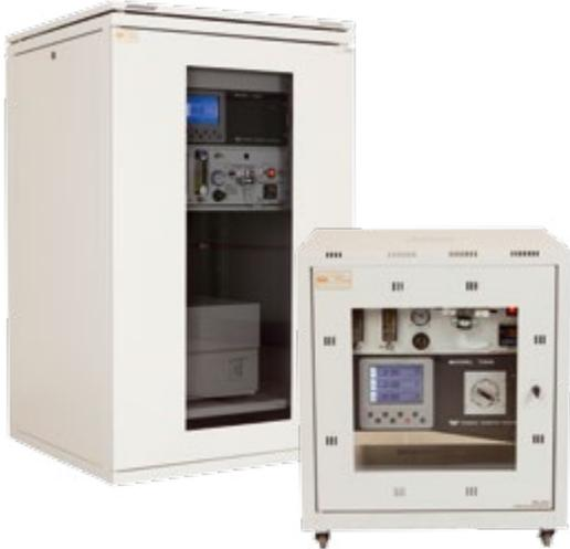
Syngas monitoring ( $\text{CH}_4$ ,  $\text{CO}$ ,  $\text{H}_2$ ) system that contains gas conditioning unit and software controlled analyzer data collection
