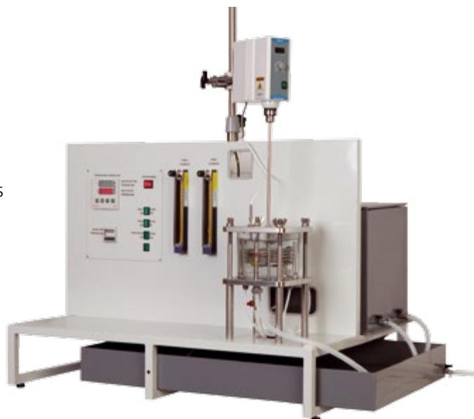
Example of a standard designed CSTR system that contains manual controlled stirring, flow rate and temperature options
