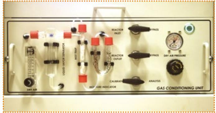
Example of a downstream conditioning unit including rate, moisture indicator, halogen scrubber, mist trap, L/V separation and membrane drying equipment
