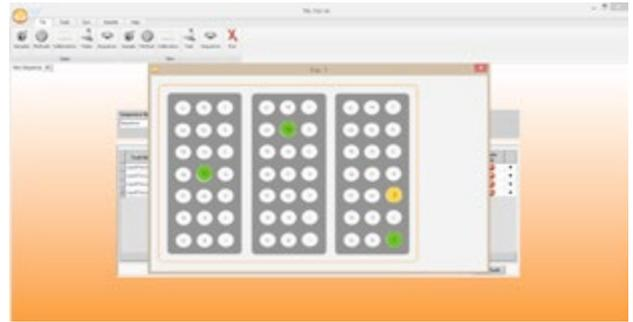
Example of Sequence development screen for Liquid Sample Autosampler with 63 vial positions
